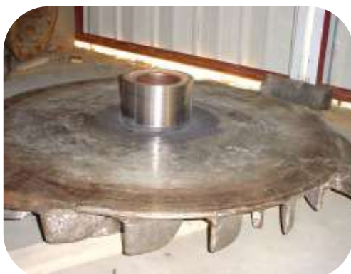
Paper Pulper badly worn and was in urgent need of repair. Surfaces were abrasive blast cleaned and rebuilt using 107 Metal Repair Paste XL.
