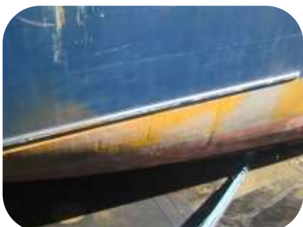
Corroded bow on large container vessel abrasive blast cleaned and filled using 101 Metal Repair Paste
