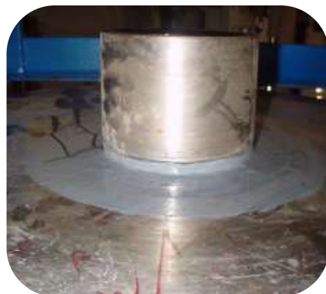
Paper Pulper badly worn and was in urgent need of repair. Surfaces were abrasive blast cleaned and rebuilt using 107 Metal Repair Paste XL.
